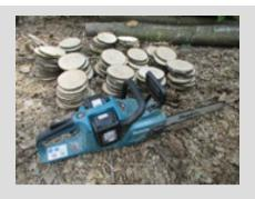
In (typical hedge laying) wet weather the Stihl battery box seems designed to collect water (does not even have a drain hole!), on one very wet day last season Marcus Broom turned his saw upside down to empty the rain out, but it was still working, with the Makita batteries sit on the outside of the machine the rain should be less of an issue, but realistically chainsaws will be used in the winter so it would be good to know from the manufacturers that we can use expensive kit outside.
